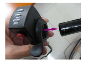
Place your hand on the bar and find the position where your thumb feels most comfortable pressing down on the throttle.
