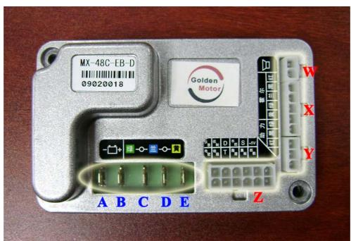
Your controller looks something like this. Notice that the controller has 5 single connectors labeled: A, B, C, D and E and 4 pin-connectors labeled: W, X, Y and Z. Usually the controller comes with wires already connected to the connectors. If otherwise, the following will tell you more information about the wires.
