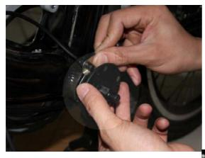
Place the outer magnetic ring next to the inner ring. Make sure they do not have any contact in between using washers.
