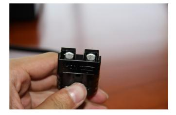
Make sure the "Nails of the Talon" has reached the end and clipped onto the metal plate. If this is done correctly, it is nearly impossible to pull out the power cord without tools.
