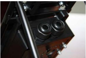
First, slide the power cable through the controller box's hole as shown on the right.
