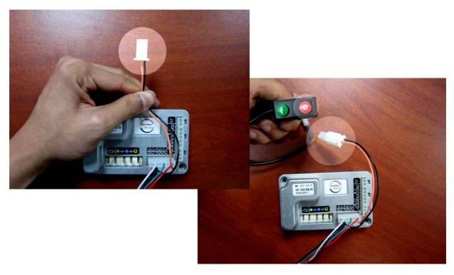
Find the 2-hole pin connector (Beige and Black wires) and plug it into your Cruise Control system.
