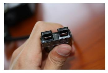
Watch out for the "+/-" signs on the connector, make sure Red goes into + and black goes into - . Push all the way in until you hear a click sound.
