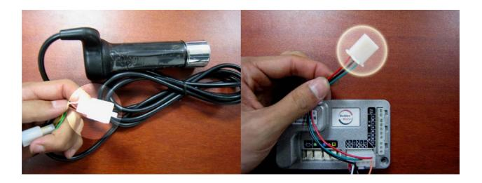
Take the throttle wire and single out the 3-hole pin connector. Take the 3-hole pin connector (Blue, Black, Red) from the controller area Z and plug them together.
