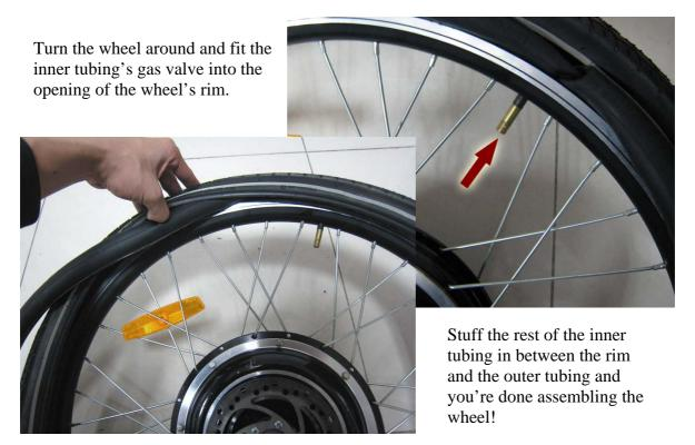
**Important Note:** Please choose an inner tube with a longer valve as Golden Motor rims are double walled. The rims are double walled to be able to withstand the powerful torque from the motor.
