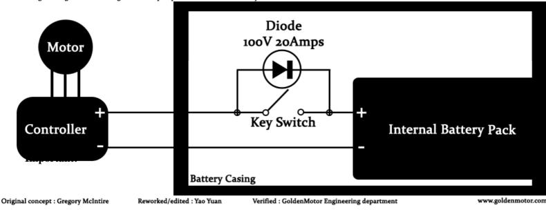
Solution Diagram: Regenerative Braking down a steep slope burns controller if battery is turned off.
