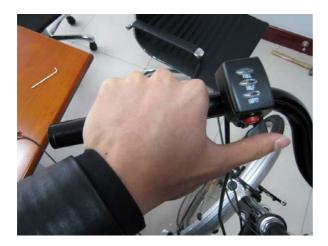
Use the 3.0mm Allen Wrench and tighten the bolt beneath the throttle.
