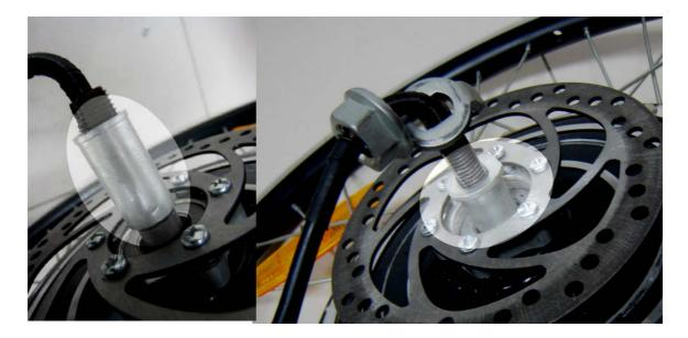
**Safety Note:** The Disc Brake Plate-Tube holds the disc brake in position. It is a very **important** component in the Disc Brake System.
