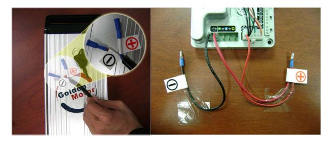
Take the Battery Pack's wires and connect them accordingly.
