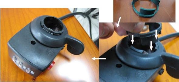
**Note:** This tripod comes useful if you are installing the thumb throttle on the right side of the steering bar. The tripod prevents the edge of the movable ring from getting stuck when it comes into contact with the exterior handle bars.
